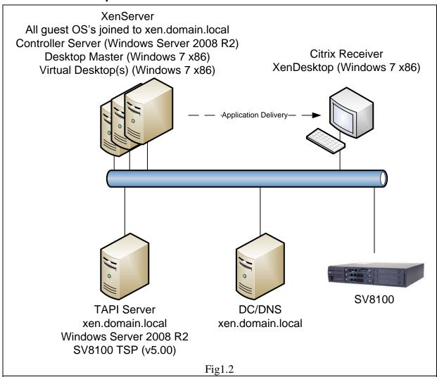
The above is the setup used to provide TAPI operation under XenDesktop.
