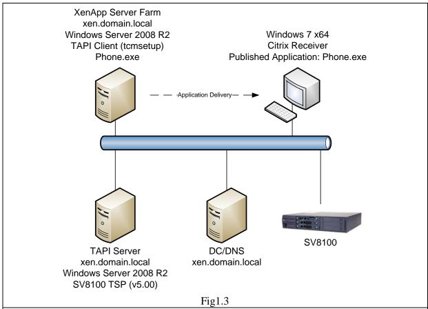
The above is the setup used to provide TAPI operation.
